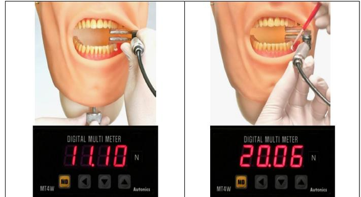
**Figure 6.** The chin screw of the manikin was tightened until reaching a value next to 20 N. This step was monitored at the digital multi-indicator panel of the dynamometer.
