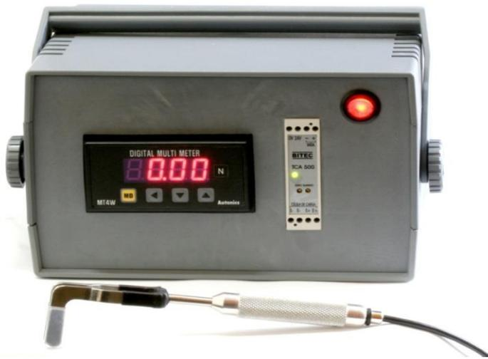
**Figure 2.** Frontal view of the dynamometer ready to perform the tests.
